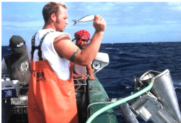
Fig. 1. The underwater setting chute delivers baited hooks while setting so that they first emerge underwater out of sight and reach by diving seabirds. The chute's slot enables external deployment of the main line, buoys, and radio beacons. The main line is set through a line setting machine, baited hooks are sent through the underwater setting chute (directly in front of the crewmember with the baited hook), and the branch line with the baited hook is clipped onto the main line moments after the baited hook is sent down the chute.
