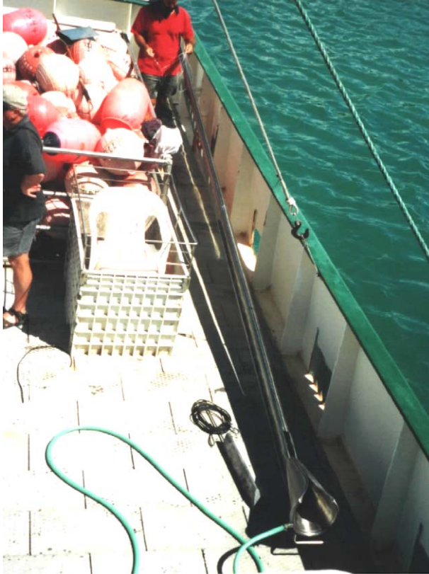
Fig. 2. The underwater setting chute is stored on deck against the bulwarks. The chute used in this trial is 9 m long and when deployed, 5.4 m of the chute's shaft is underwater.
